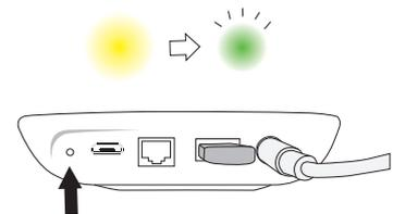
**c** The gateway starts to restore data, and the indicator light will rapidly show a series of fast and slow flashes of yellow and green lights. When the indicator light turns to steady green light. (This takes about 3-5 mins), the gateway has restored the data successfully. (If a red light appears during this process, the recovery has failed, please check whether the backup data is valid)
